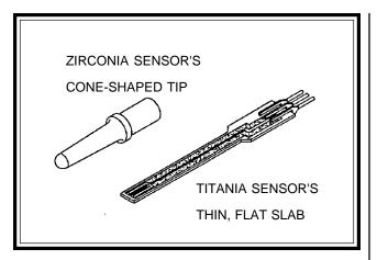
changing an 02 sensor. The two look very similar, but *are not interchangeable*. The connector is even the same on the Titania and Zirconia sensors on some Jeep models.
