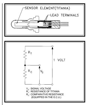
In the case of the three-wire Titania sensor, the reference voltage is supplied from the heater circuit. The heater circuitry is designed so that one volt is left after traveling across the heater. This one volt then becomes the reference voltage that goes across the resistive Titania. (Fig. 2)
