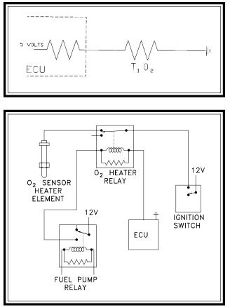
Since this five-volt signal comes from the computer through a comparative resistor, then across the Titania, the computer will see different values for rich and lean. When the system is rich the computer will see 0 to 2.5 volts. When the system is lean the computer will see 2.5 to 5.0 volts. (Fig. 4)
