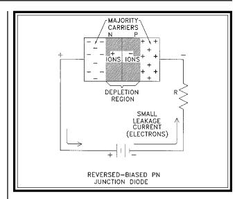
PN junction where they will combine with some of the holes and an extremely small current will be produced. (Fig. 7) This is typically microamperes in germanium diodes and nanoamperes in silicon diodes.
