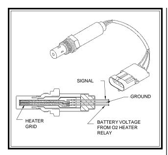
This results in a high voltage signal to the computer.
