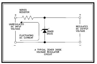
The most widely used application for a zener diode is to continuously reverse bias the diode, so it constantly operates in its breakdown voltage. A zener diode used in this manner can provide voltage regulation. This voltage regulation is often required for solid state circuits that need a fixed DC voltage to operate properly.
